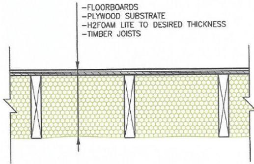
**Diagram 2 - Suspended timber floor - application from above detail**
